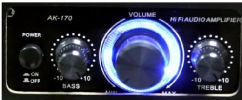
Your machine's sound amplifier controls are accessible inside the front access door of the cabinet. The sound can be switched on or off with the button on the left. The main volume dial will be illuminated when switched on.
