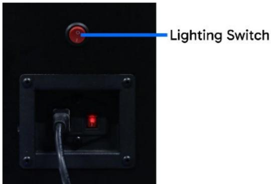
This ArcadeMAX machine includes lighting on the underside of the cabinet that can be turned on or off depending on your preference. Flip the lighting switch on the back of the machine to switch the lighting either on or off.
