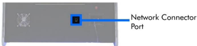
To connect the machine to the internet via a wired connection, plug a network-connected ethernet cable into the back of the machine into the Network Connector Port until it clicks. You'll be online and ready to start downloading games.
