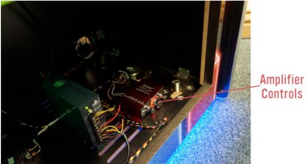
The amplifier controls can be just inside of the machine as seen above. The large central dial changes the volume, and the smaller dials will alter the bass and treble respectively. The amplifier can be switched off completely using the push-button the left of the dials.
