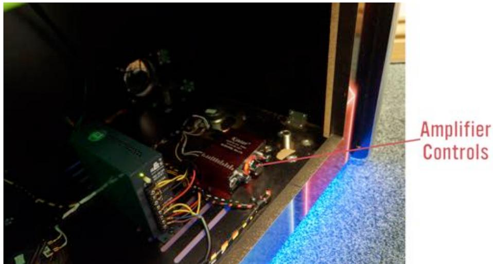
The amplifier controls can be just inside of the machine as seen above. The large central dial changes the volume, and the smaller dials will alter the bass and treble respectively. The amplifier can be switched off completely using the push-button the left of the dials. When done, you can simply close the door and lock up again.
