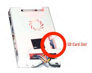
The SD Card on this system can be found on the main Pandora's unit as shown above (inside the console cabinet).
