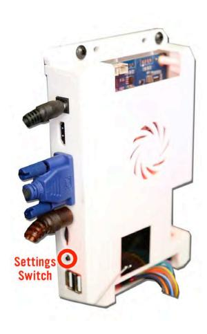
To access the options on your unit, open the access door on the back using the machine's included key and locate the main PCB unit inside. Press the small Settings Switch as illustrated.
