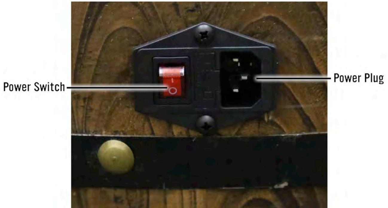
Set the ArcadePro Barrel up by plugging the included power cable into a wall socket, and then into the power plug on the side of the machine.
